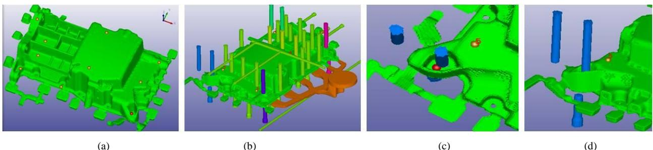
Fig. 3. Cast-Designer (a) Production sensor defines (b), (c) & (d) Define sensor attached to the cooling channel
